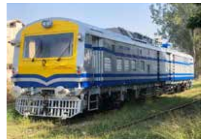
8-Wheeler Diesel Electric Tower Car (DETCIS)
