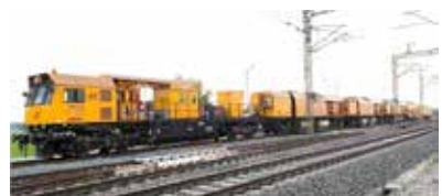
Mobile Rail Grinding Machine
