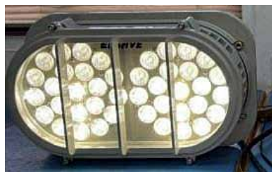
Improvement of high glare in based LED based twin Beam Headlights used in Electric Locomotives
